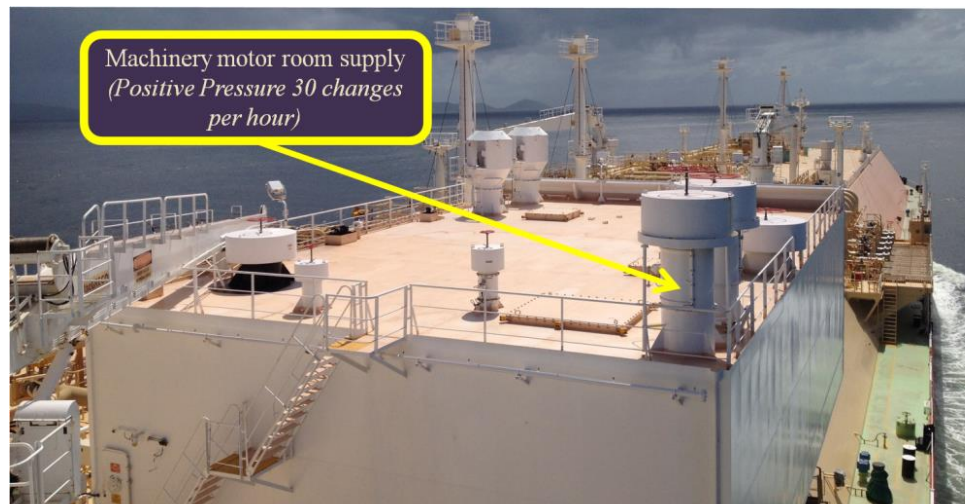
Figure 13-1 Machinery motor room supply
