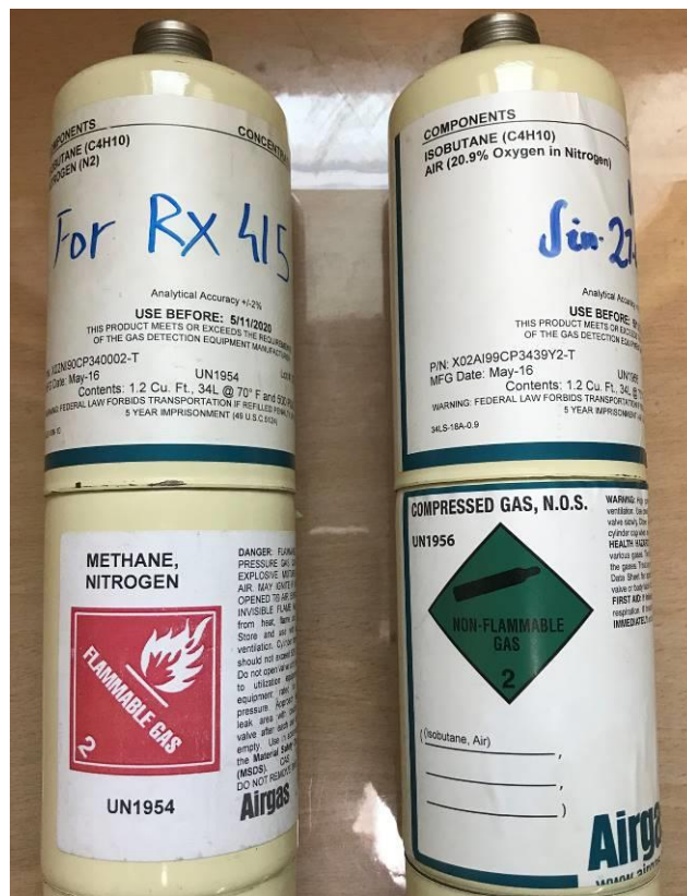
Figure 9-12 Example of flammable gas stickers
