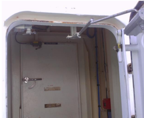
Figure 5-5 Self closing mechanism, door open, and door closed indicator
