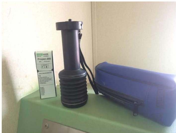
Figure 9-15 Portable gas meter
