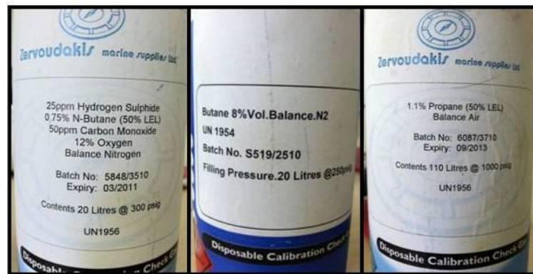
Figure 9-4 Example span gas: 4 gas; 8% butane, balance nitrogen; 50% LEL
